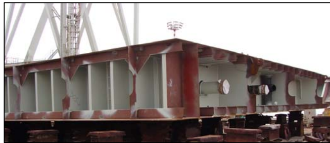
Fig. 3.54. Typical double bottom block [29]
